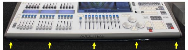
Lift front panel up and secure it using the panel stay.
