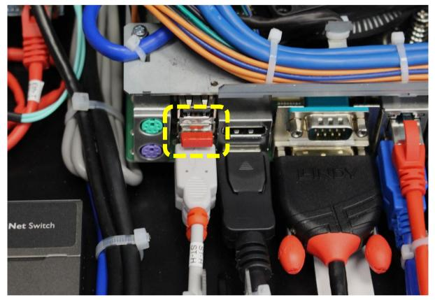
Close the unit using retained fixing
